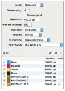
Engraving parameters and output quality control in one application
